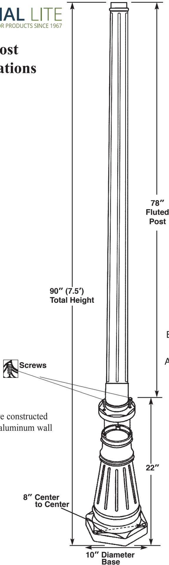
Special Lite posts are constructed of a minimum .075 aluminum wall thickness.
